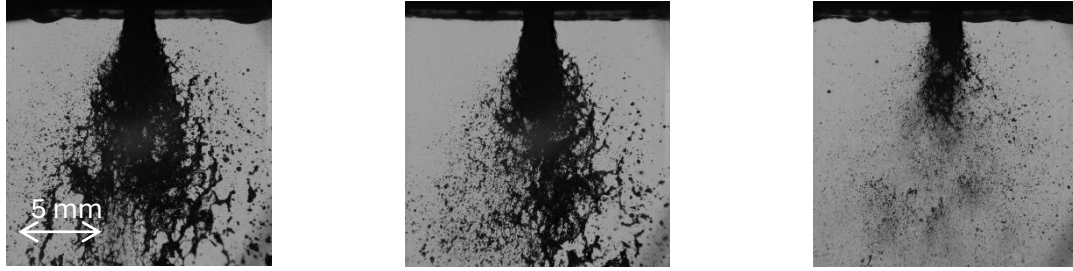
Figure 4: EFI5 side view with (central liquid configuration) for GLR = 2.5, 5 and 10\%
