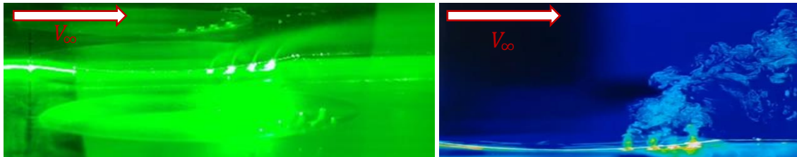
Figure 5: TR-PIV continuous blowing (left) and synthetic jet (right) visualization pictures: for better clarity, a case with a higher discreteness of holes (4 instead of 9) is shown
